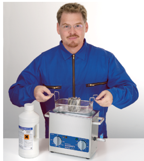
drill head cleaning in the ultrasonic bath RK 102 H
