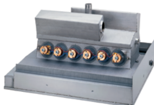
foulard ponds for sonication of dye baths
